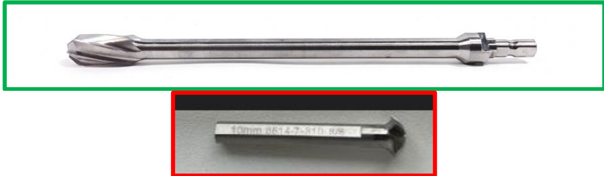
Figure 1: As labeled, conforming part 1806-2012 (top/green), and non-conforming part 6514-7-310 (bottom/red)
